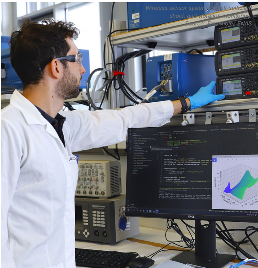
Lab setup for computer-assisted real-time measurement of impedance in a lithium-ion battery cell to analyze its state. Source: Fraunhofer IFAM
